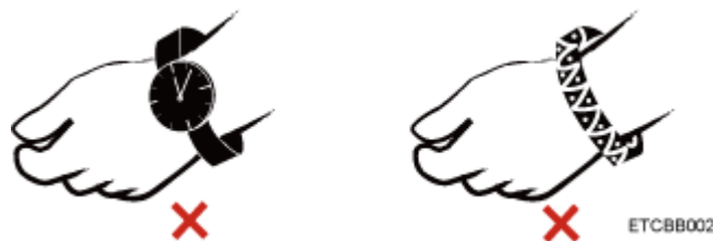
Figure 8-2 Removing conductive objects
