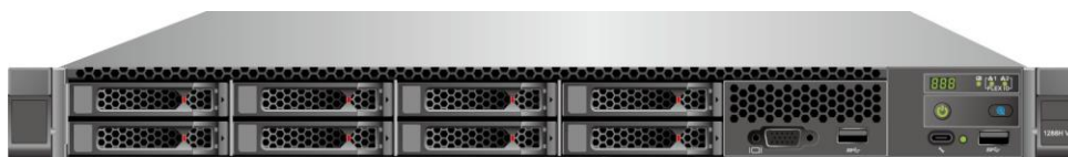
Figure 1-1 R100 with 8 x 2.5" drives (example)
