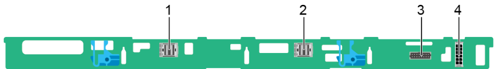
Figure 5-34 4 x 3.5" drive pass-through backplane
